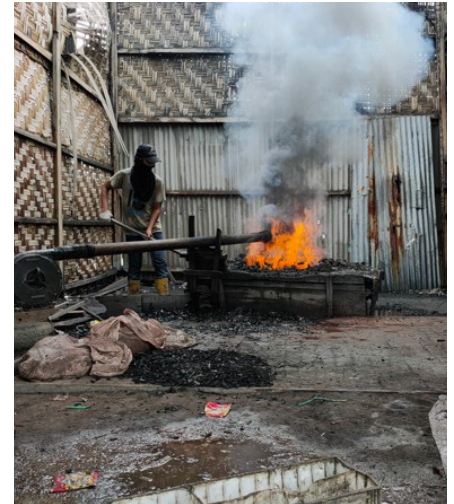
Informal backyard smelters like this one in Indonesia, are used to melt and extract lead from used lead acid batteries, releasing toxic lead-contaminated fumes and dust into the atmosphere. Image source: Vital Strategies
