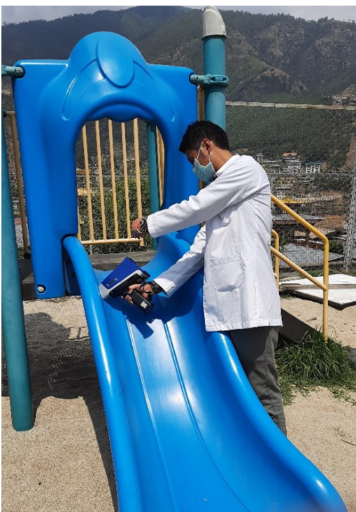
A Bhutanese researcher uses an XRF monitor to test for the presence of lead in playground equipment.
